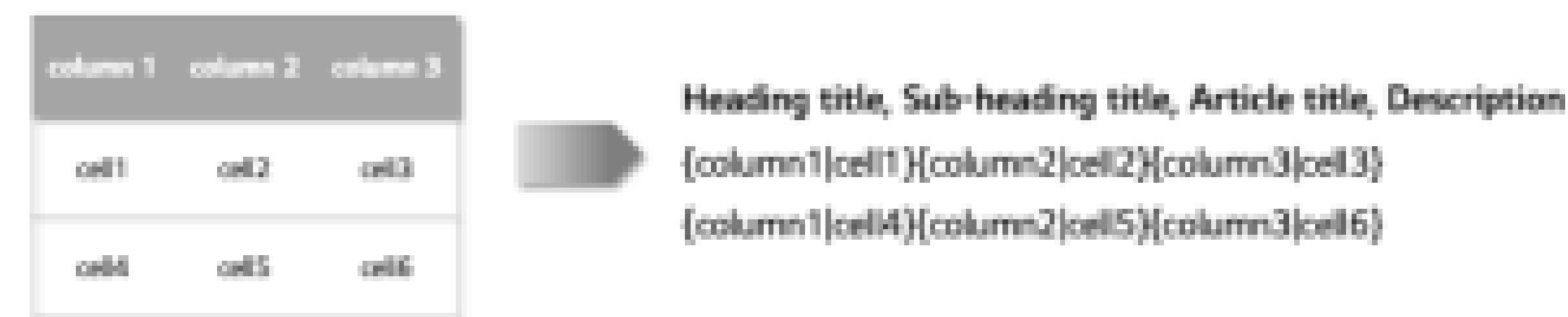
Figure 2: Converting WikiTable format into string sequences for pre-training input. The converted table strings are added with descriptions for the Wikipedia article.
