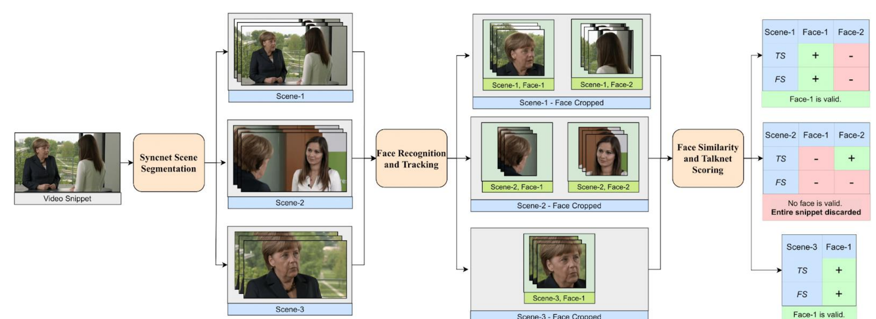
Figure 1. Speaker Diarization Pipeline for semi-automatically differentiating speakers and tuning in on one target speaker in collections of multi-speaker videos based on a few examples of the target speaker.
